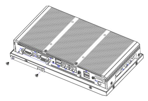
**Step 1.** Unlock 2 screws from the rear side of the panel PC as above.
