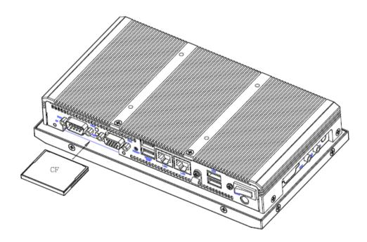
Step 2. Put the CF card into the socket and fasten 2 screws back.
