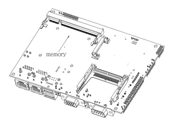
**Step 3.** Insert the SODIMM into the memory socket.
