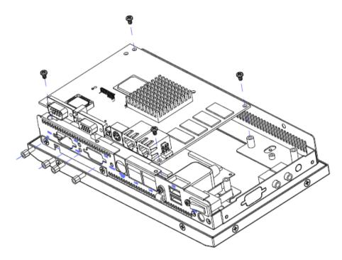
Step 2. Remove 8 screws as above and have the box pc and board separated.
